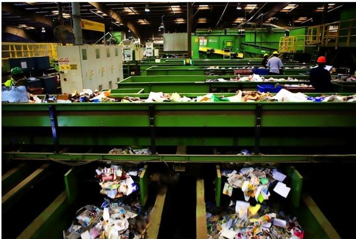
residential programs throughout the Hampton Roads region. State of the art when originally installed, the MRF has undergone substantive renovation and upgrades throughout 2017 and 2018 and is one of the most automated mixed materials recovery facility in the United States. It is engineered to process up to 40 tons of materials per hour.
