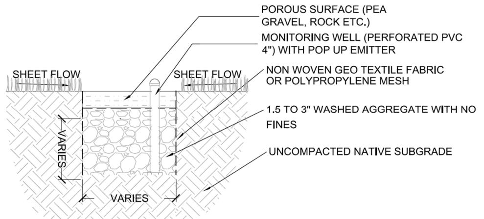
**Typical Infiltration Trench Cross Section**
