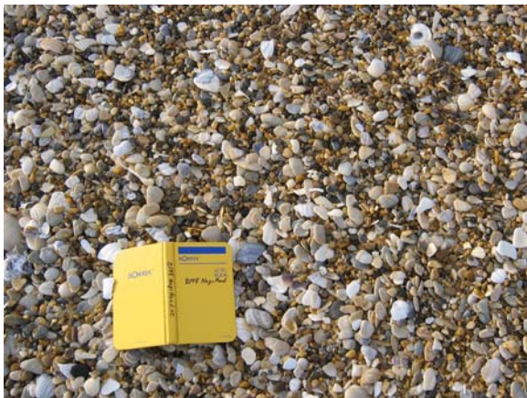
FIGURE 21. Nags Head beach samples span a wide range of sizes both cross-shore and alongshore, making selection of the “native sediment” size subjective.
