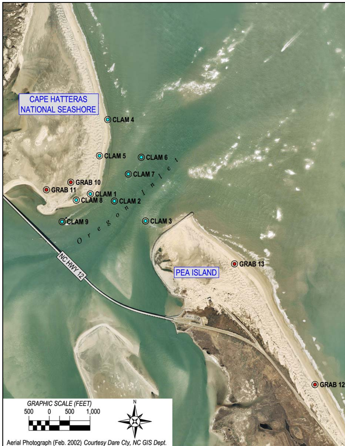
FIGURE 27. Oregon Inlet and Pea Island showing general location of sediment samples obtained for the present study.
