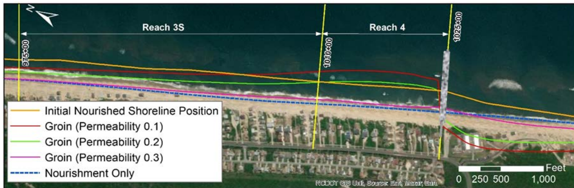
Figure 7-7: GenCade Shoreline Modeling Results for Terminal Groin Alternative.
